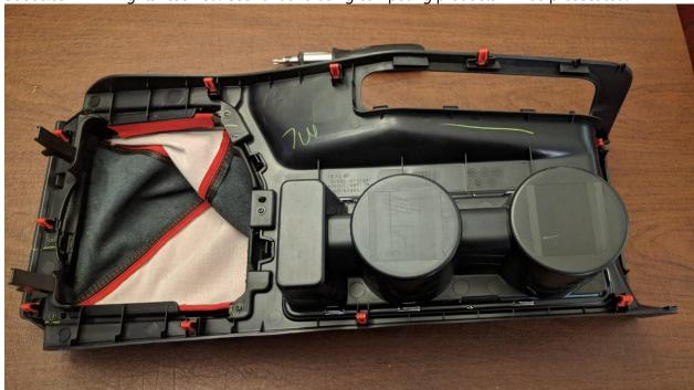
Replace the ebrake boot (see below) if you bought a RedlineGoods one, or just reassemble the console back into the vehicle. Use a little blue loctite to secure the gear shift knob correctly aligned and taught. Be careful to not drop the blue loctite onto the gear shift boot. Reattach the shift knob and enjoy!
