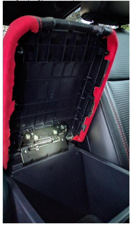
Install the armrest inner cover with the 6 small phillips screws
