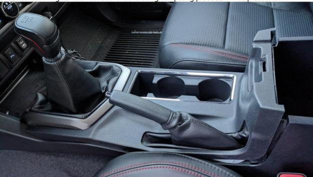
Remove the gear shift knob by grabbing the chrome ring between the boot and the shift knob, and twist it counter clockwise. Unscrew the the shift knob.
