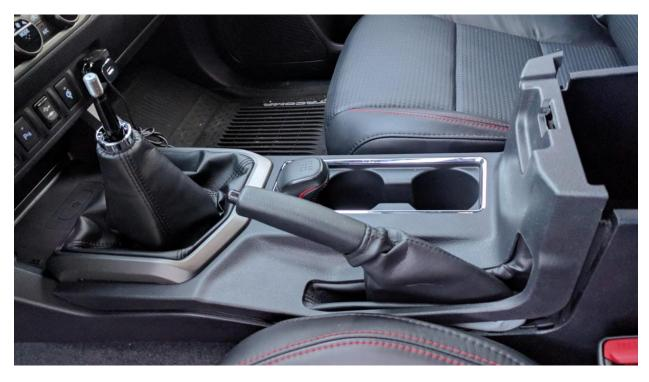
Continue to lift the center console cover over the gearshift lever and handbrake handle. Depending on vehicle equipment you might have to disconnect an accessory connector before the console can be removed from the vehicle completely, so don't pull on the console too quickly.
