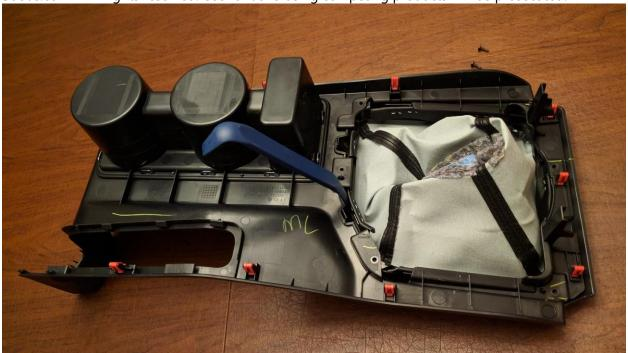
With the shifter mounting bracket separated from the console cover, remove the shift boot from the trim cover.
