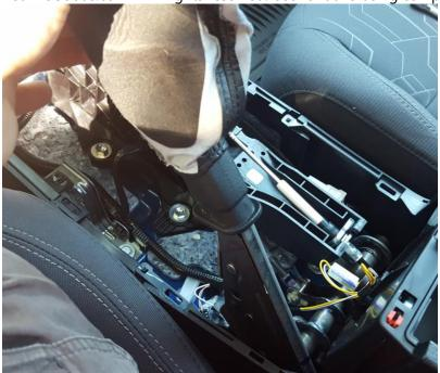
Pull trip panel upwards and off the e-brake lever. (E-brake lever should be in full on position)
