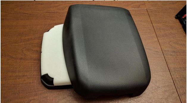
Install the new cover onto the armrest. The new cover needs to be glued.
