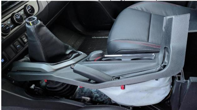
Now that the center console cover is completely removed, you can take all the parts to a work bench/table to continue with the removal procedure.
