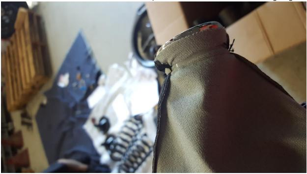
Remove the factory boot material from this plastic mounting bracket. It's glued on, so force may be
