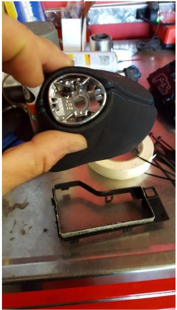
Once the adhesive is dry to the touch, remove all the tape and mate the leather boot to the trim ring. Remember this shift knob colar points forward! Also pay attention to the seam alingment. You may want to test fit the pieces into the console before you glue them to mark orientation with a piece or chalk or crayon. Take your time!
