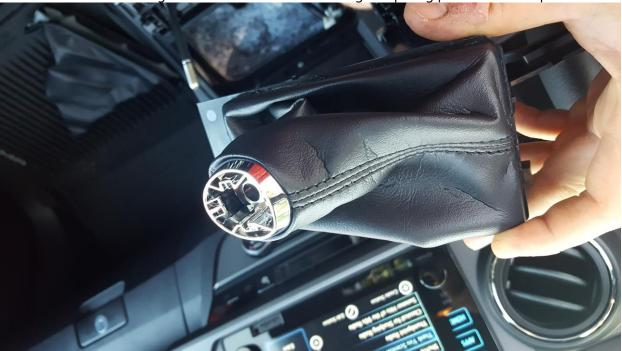
Turn the shift boot inside out and cut this zip tie. Remove the chrome mounting ring collar and save.
