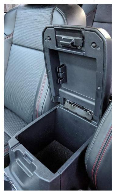
Use a trim removal tool to pry open the top of the armrest from the inner cover that was held by the 6 screws just removed
