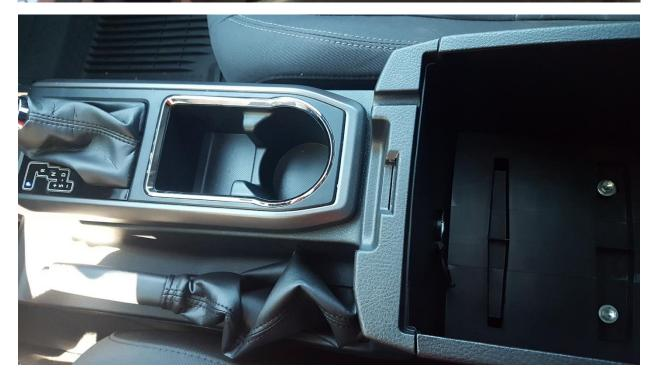
Screw the factory shift knob back into place and pull up on the shift boot trim ring to snap it back into place.
