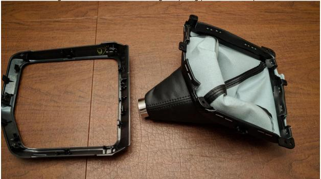
Flip the shift boot inside-out and cut the tie-wrap holding the collar in it.
