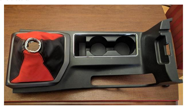
Check that all 12 red trim clips of the center console cover are present and securely fastened before reinstallation back into the center console.
