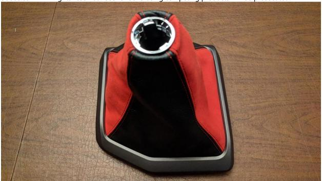
Re-install the shift boot along with the shift boot trim to the center console cover using the reverse of the removal above.
