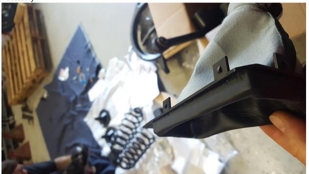
Take your new leather boot and turn it inside out. Slide the plastic collar inside (upside down) with the narrow end pointing forward and zip tie the leather boot to the collar like so.
