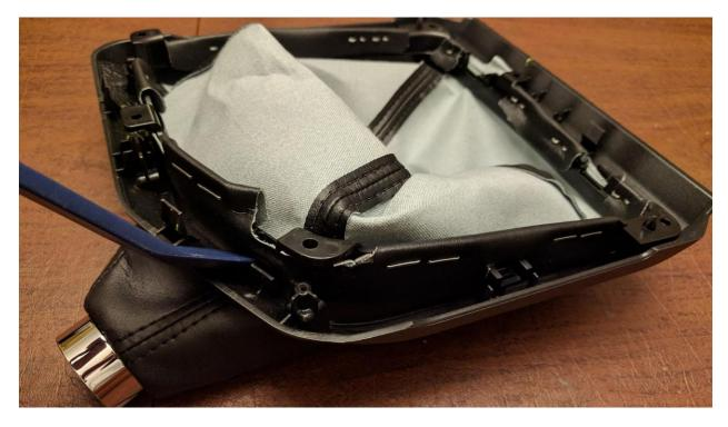
Remove the frame and unstaple the boot from the bracket.
