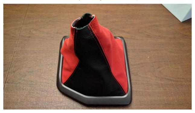
With the diagonal edge of the shift boot trim closest to you (same orientation as when it is installed in the vehicle), fold the top edge over, and mark the center of the top edge furthest away from you (edge that points to the front of the vehicle)
