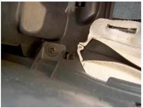
There are 8 philips head screws to remove inside the consol, these allow the bottom party of the console to lift. The outer edge of the boot is held between the two parts of the console.
