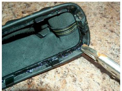
It may be necessary to use clamps the hold the leather down to the plastic. Then let dry. Reinstallation is reverse of removal. Open Velcro on the new boot and slip over shifter. Press the base of the ring down until you hear and feel it click. Wrap Velcro back up under the shift knob and reverse lock and your new shift boot is installed.
