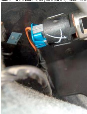
The 12v plug on the passenger side of the console must be unplugged before the console can be fully removed. There is a clip onteh front side of the plug to push in to unplug it.
