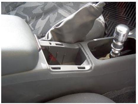
Start to lift the console, as you work it up, continue to slide the brake boot up the handle.
