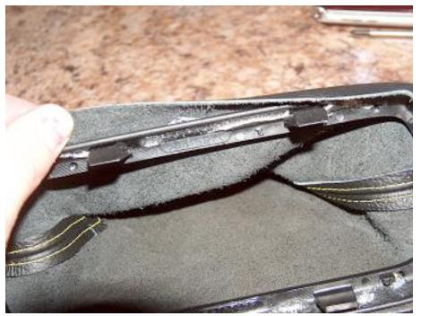
Run a seam of plastic adhesive along the outer edge of the ring to adhere the boot.
