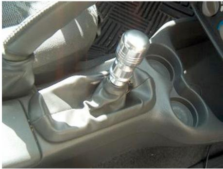
Note the car in the images has had a short shifter installed. The stock shift knob is removed by twisting counterclockwise but removal is not necessary for boot replacement.
