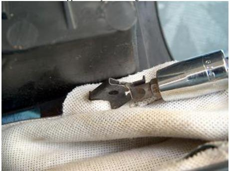
On the inner side of the boot there are two metal clips holding down the boot leather and retainer, use a flat blade screwdriver and carefully remove these. Don't use too much force the plastic they are attached to is thin and breakable.
