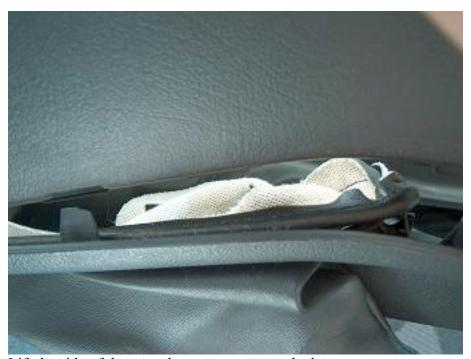
Lift the side of the console apart to remove the boot.
