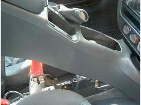
Pull the console off the rest of the way. It takes a bit of working around but don't force anything.
