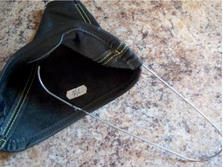
The new boot has 4 slots cut into it, pick one to begin to slide the ring into the seam.
