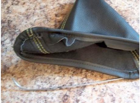
Work it around carefully, trying not to push it through the thread or through the leather. Once you have the ring completely inside the bottom seam of the new boot try to shape the wire back to it's original shape with the vertical seams in the middle of each bend.
