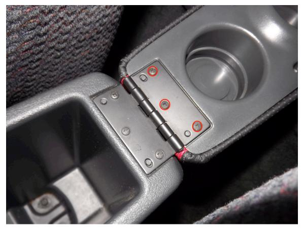
Remove the armrest and then unscrew the four circled screws. Pull out the plastic piece that this releases.
