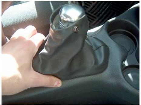
The boot can then be removed without removing the shift knob and will slide over top. Squeeze the base of the shift boot lightly and push it forward to lift it off the console.
