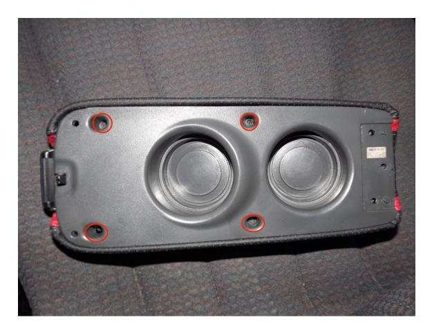
Pry off the staples holding the stock armrest cover to the plastic. A combination of needle-nose pliers and a flathead screwdriver work well here. Once all staples are out, rip the cover off (it will be held to the top by glue).
