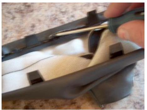
The stock boot is glue to the ring that holds it down to the consol. Use a flat blade screwdriver or knife to pry it away being careful not to damage or crack the plastic ring.
