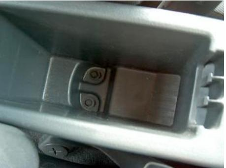
Remove the four 10mm bolts from inside the console, under the window switch and in front of the cup holders.
