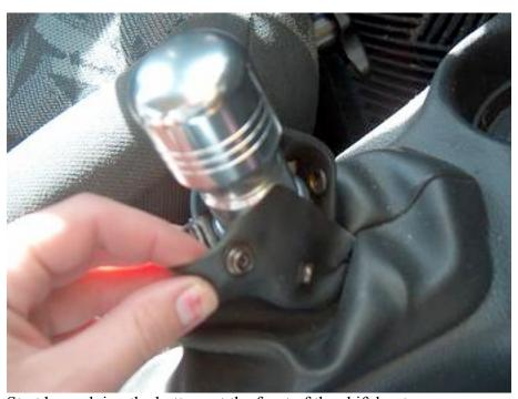
Start by undoing the buttons at the front of the shift boot.
