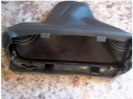
Once the ring is free from the old boot fit your new boot around it. Center your seams and bring the bottom edge of the boot so that about 3/4 of a cm will wrap around.
