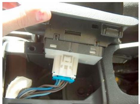
Push the clip on the side of electric plug in to unplug it and set switch aside.
