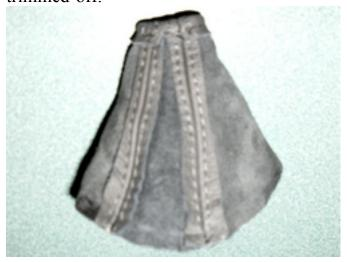
Turn the shift boot inside-out, then take a small, sharp pair of scissors and cut off the extra seam material as close to the stitching as possible, while leaving enough material to adequately support the stitching.
