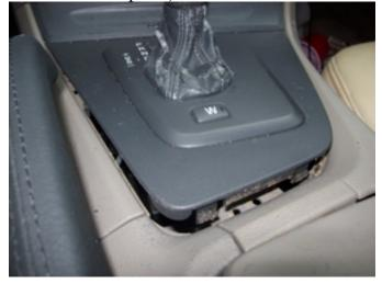
Now, separate the smaller inner base plate from the outer base plate by depressing the four small tabs in each corner of the base plate.
