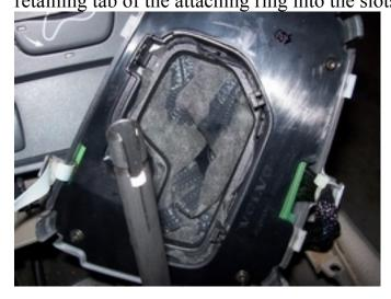
Even though we trimmed off the excess leather, the collar will probably still need a little bit of pushing and prying to get it to go all the way into the inner base plate. You might have to pull up on the leather at the same time to insure that it's not binding on anything, but is settling into its normal position. Finally, make sure the four feet on the bottom of the collar are wedged securely into their retaining holes.
