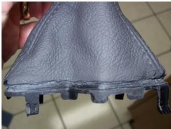
The old boot was attached by seven small tabs or ears, which were inserted through equally small slits in the original imitation leather shift boot. The new leather boot did not come with any pre-cut slits to receive the tabs. Redline may have logically reasoned the slits would be more accurately cut on site, with the
