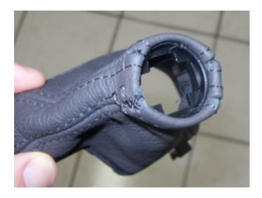
Last, but not least, the stiffness and thickness of the leather boot causes the base plate assembly (inner and outer) to shift forward (and squeak) when we put the gear shifter into Park
