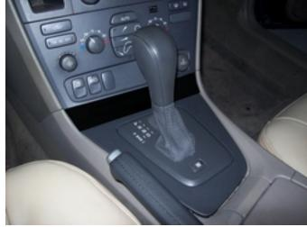
Insure that the ring is locked in place all the way around the bottom of the shift knob. Sometimes it seems like it is locked in place, but only half of the tabs are fully seated in the slots. There should be no gap between the boot and the shift knob, or at least only a very small gap, which will later be remedied with a little silicon adhesive/sealant.
