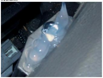
Now, push the base plate assembly down into place again, but this time the silicon (once it dries) should help lock the base plate assembly to the post and the shelf, and offer a slight cushioning effect. Clean up any excess silicon. Be careful not to use too strong of a solvent when cleaning, as it can damage the paint on the plastic.
