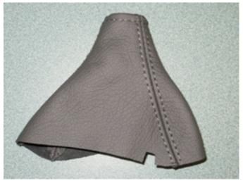
This notch lines up with one of the four feet on the attaching ring. This particular foot sticks out further than the other three
