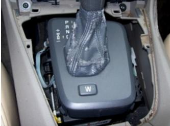
Insert a small flat-headed screwdriver between the top of the shift boot and the bottom of the shift knob.
