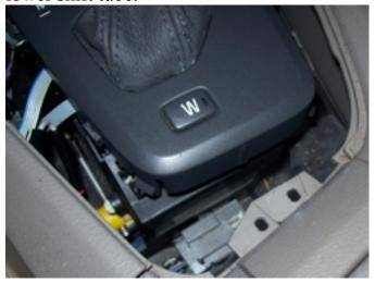
Make sure the small round plastic ring is still attached to the top of the boot, as you slide the boot over the lower shift tube, and that the wires below the inner base plate are neatly tucked underneath, including the black wire loom that hooks back into its clip on the right-underside of the shifter.
