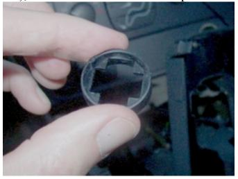
This ring must be pried slightly outward and then down. To do that, you have to get your screwdriver behind the ring and carefully pry it out and away from the shifter shaft just below the shift knob. If you work at it a little bit, the ring should release from its holding tabs, and the top of the shift boot will slide downward.
