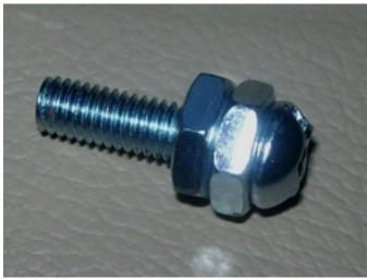
Insert the screw (with the two nuts) into the right side (or passenger side) hole, and secure it with two additional nuts under the bottom of the plastic shelf.
