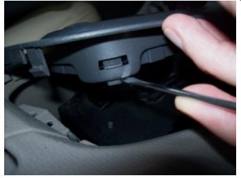
Actually, if you can get three of the four tabs loose, the fourth one will drop right out. Here's another tip: do the right front tab first, then the rear two tabs.
