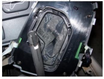
Locate the four tabs on the attaching collar, and pry them away from the inner base plate, one at a time, to separate the collar from the base plate.
