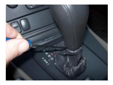
There is a small round plastic ring (about one inch in diameter, and about 3/8" tall), which is located inside the top of the shift boot, just below the shift knob.
