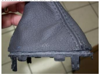
So, how and where do we mark the boot for cutting? There are two ways to do this: The first method is to position the boot on the collar in the desired position, and mark the boot all of the way around at the approximate position of the bottom corner of the "L" (as if the boot were going to fit down as far as it could go without going over the step). By the way, you will find it much easier to mark the boot (and to see the mark) if you purchase a pen with white ink.
