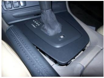
This happens because the extra thickness of the boot creates a slight log-jam effect when the shifter tube, in its travel to the Park position, gets close to the front of the inner base plate, thus causing the shifter tube to actually push against the inner base plate, via the folds of the boot.
