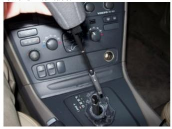
However, it will require a good deal of upward force to get it to move. When this happens, and the shift knob assembly comes flying out, you will likely think you have broken something. Don't worry, it's not damaged, and should go back together perfectly well. Once it breaks loose, it's out instantly.
