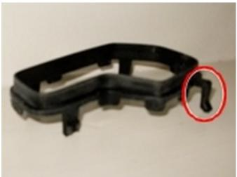
so you will know right away that this foot fits inside the notch, and you will also know how to orient the shift boot on the attaching collar, including its depth.
