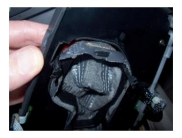
Once this is done, remove the collar (with the boot) from the base plate.
