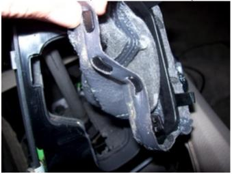
Pull the shift boot away from the attaching collar by unhooking the boot from the seven small retaining tabs on the collar. The tabs protrude through holes in the shift boot, and separate easily.
