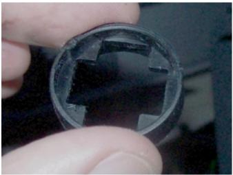
There is a problem here, however. Again, because of the thickness of leather, the ring will not fit into the boot and function as it did with the original thin imitation leather boot.
