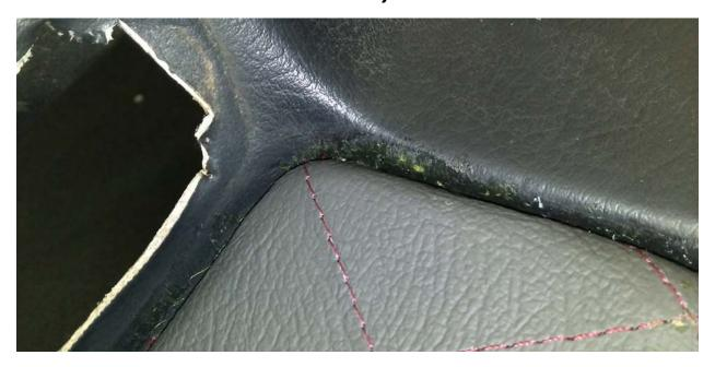
The best technique to remove any existing adhesive is to rub it off of the vinyl with your bare finger. Do not wait a long period of time to do this; you will not be able to remove the adhesive from the vinyl very easily if you wait an extended period of time. You can use a dull scraper or tool to "rub" the adhesive out of the crevices as well. Be careful not to damage your vinyl.
