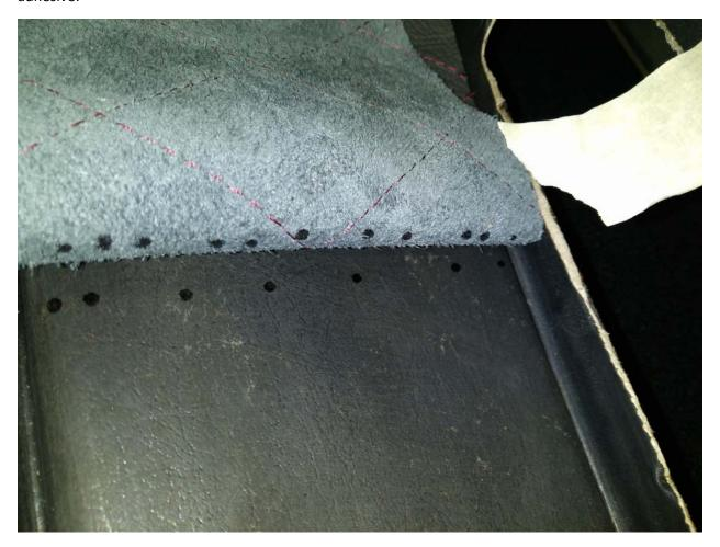
If you make a mistake then you do have a short window of time to pull the insert up and reposition. If you do end up repositioning, then you will need to reapply the adhesive. Pulling up the insert requires a firm and abrupt "jerking" motion; if you apply gentle pressure then you make not accomplish anything except pulling up the vinyl that is on the door panel.
