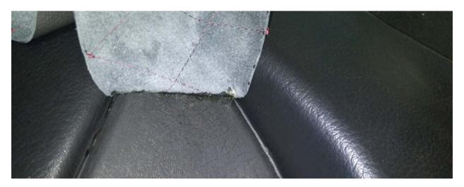
After the corner is applied properly, you can then pull up the rest of the door panel do it in sections.
