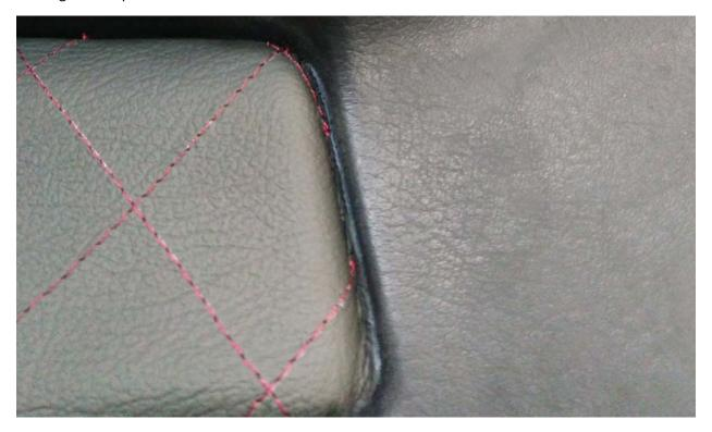
Once trimmed, attaching the piece is just like the rest. You apply adhesive to both sides, wait until tacky, and then press down the insert onto the surface and into the crevices.
