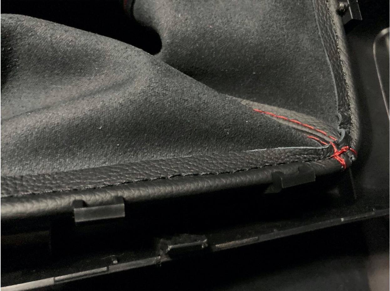
**8. THE SHIFT BOOT CONSOLE JUST POPS BACK IN TO PLACE, PUSHING ON EACH OF THE CORNERS CAREFULLY.**
