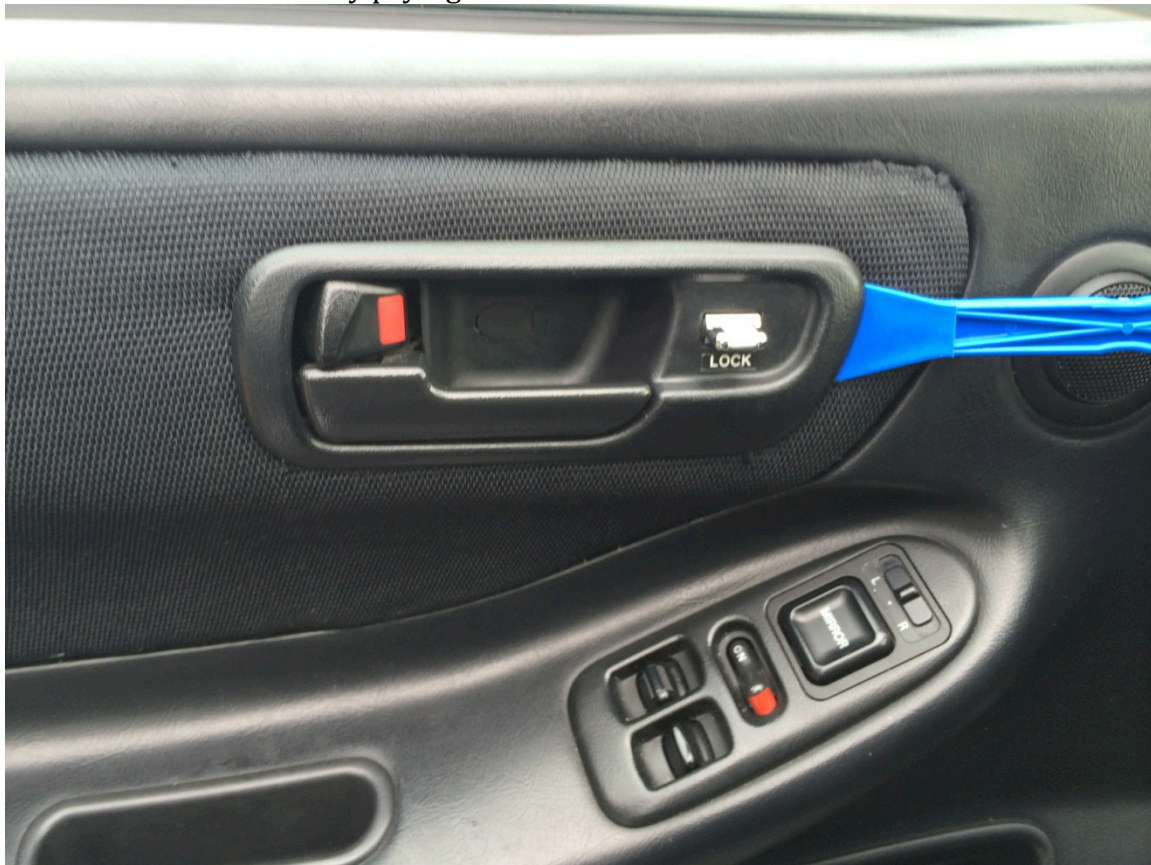
C: Remove door handle by prying from the side
