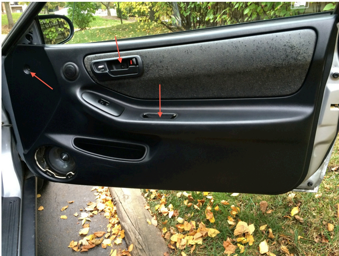
C: Remove door handle by prying from the side
