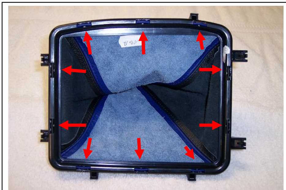
Figure 7a. Redline boot fitted on retaining ring.
