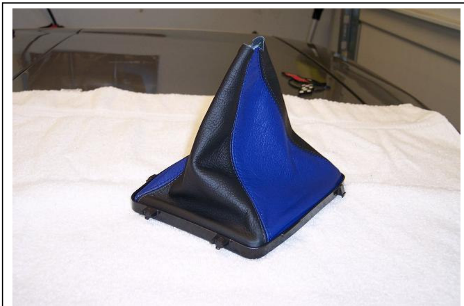
Figure 7c. Redline boot installed on factory retaining ring.
