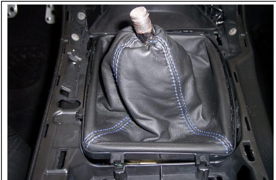
Figure 5b. Aftermarket threaded knob removal. Threaded shaft shown.
