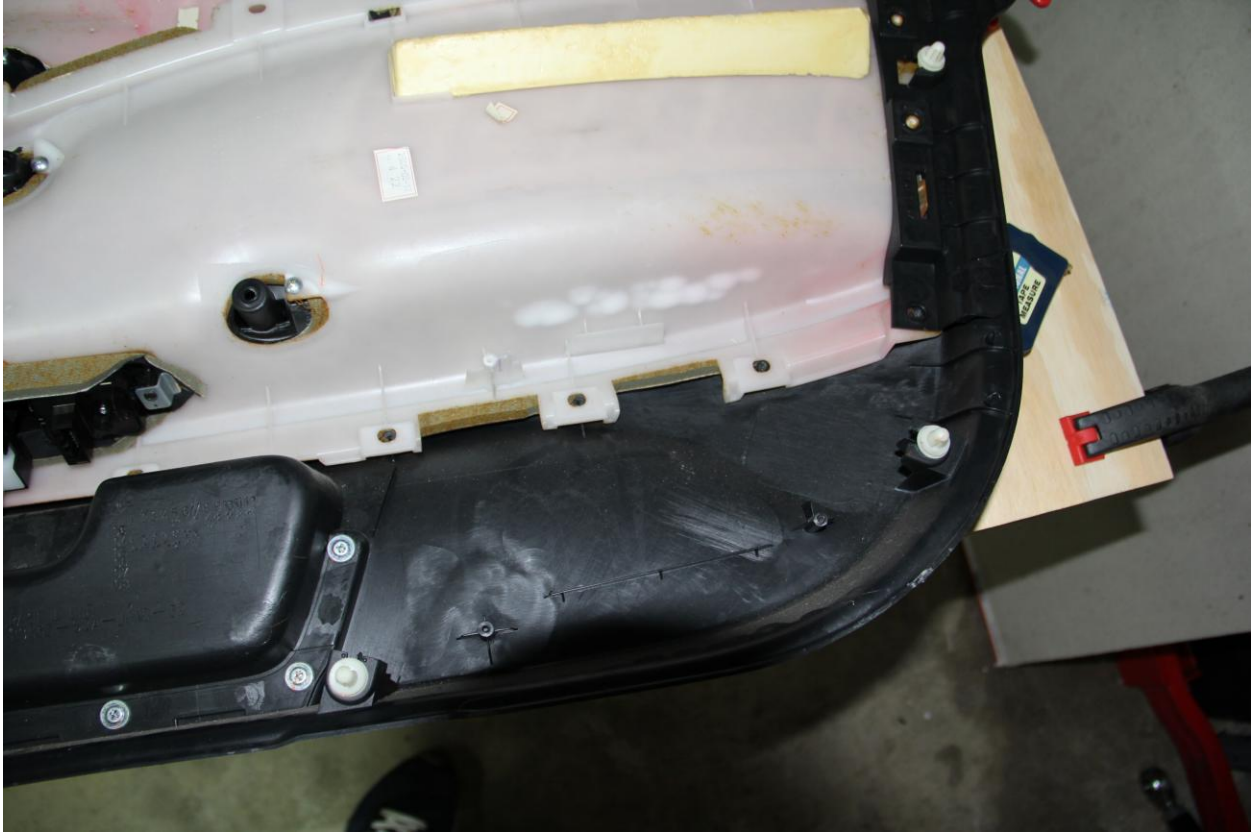
Figure 10 – The 6-sided plastic support must be removed to access one of the door card screws
