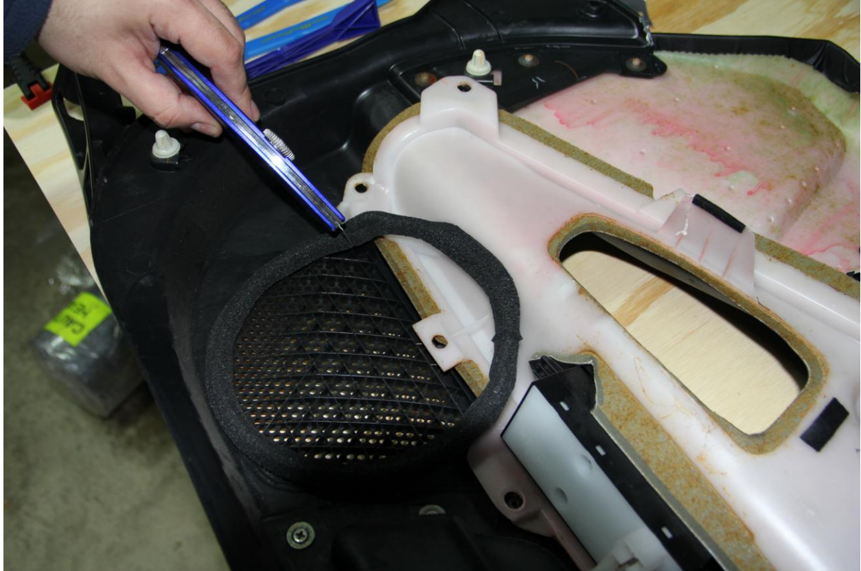
Figure 11 – cut the speaker foam to separate the door card from the panel
