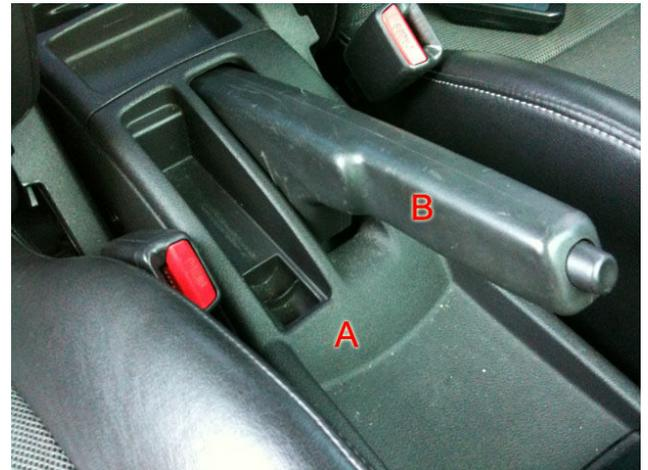
**Step 2:** Cut the e-brake handle cover as shown and discard the front portion as it will not be needed for this installation.
