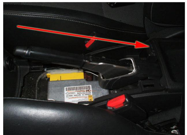
**Step 4:** Cut and discard the plastic piece on top of the e-brake mechanism using a razor knife. Use the knife to shave the raised plastic portion of the handle down until the MOMO handbrake handle fits snug. Test for snug fitment often as you shave down the plastic to ensure you don't remove too much.
