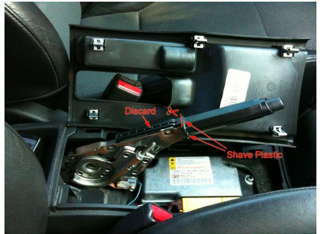
**Step 5:** Remove the black plastic retainer on the end of the e-brake handle. Invert the e-brake boot and place the e-brake handle inside of the boot as shown. Ensure that the bottom of the e-brake handle is in line with the single lower stitched line on the boot. The top of the handle should be centered between the two upper stitched lines on the boot. Use a zip tie to hold the boot firmly in place.
