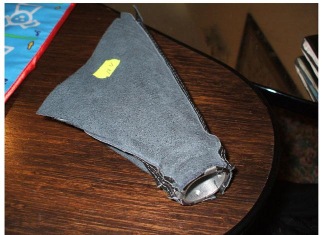
**Step 6:** Re-install the e-brake bezel and new boot / handle combo by placing the shifter knob back into 3<sup>rd</sup> gear and pulling the e-brake as high as it will extend. This will allow you to mock the bezel in position as shown and tighten the locking screws for the MOMO handle. If the leather boot is blocking the screw holes, use the razor to remove the area that is blocked. Be sure to align the boot properly before snapping the bezel back into place.
