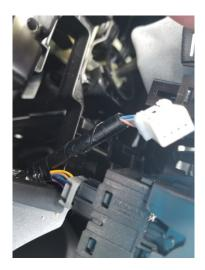
Once you get the center piece free, you will need to disconnect the electrical plugs, 2 on the left side, and 1 on the right side. Each plug has a small tab that you push in to release it. Then you should be able to pull the whole assembly off, if you have an aftermarket spacer like I have you will have to cut the zip tie attaching your shift boot to it.
