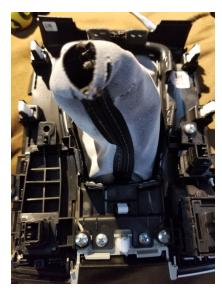
Next you will need to remove the electronic switches from the shift boot assembly – there are two screws holding each one on so remove the four screws to get them loose from the assembly.
