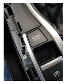
There are two screws on either side under the brackets you removed, remove them, then take a pry tool and start at the bottom to begin popping loose the clips that hold the center piece in.
