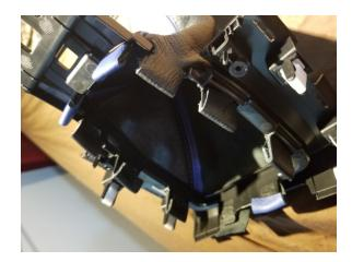
Pull the tabs on your new custom shift boot through the slots – You can use glue or double-sided tape to hold them in place.
