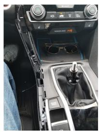
Then use a screwdriver, or plastic pry tool, to get the two side pieces off. Start at the bottom by the parking brake and pop the clips upward, be especially careful on the top clips by the climate control (They are at an angle) – when replacing side pieces start at the top and pop the clips in)
