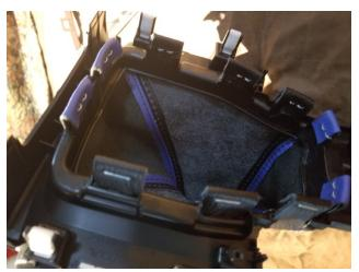
Now you can go around and staple the 10 tabs into place to secure the shift boot – you will have to use a somewhat heavy duty stapler for this to go through the leather and plastic tabs.
