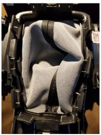
Go around to all 10 staples prying up the ends, then you can remove them. After removing all the staples, you will find a small bit of adhesive holding the tabs in place, pull them away from the adhesive, then you should be able to pull the shift boot out of the assembly.
