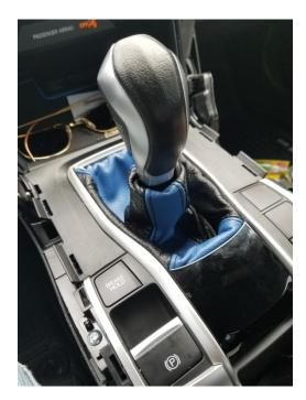
Reassemble your dash, you will need to attach the shift boot to the shift knob you are using – mine had a nut that used a zip tie to secure it to the shifter. You may have to spin the entire assembly, with your shift knob, onto the shifter rod before reassembling your dash panel.
