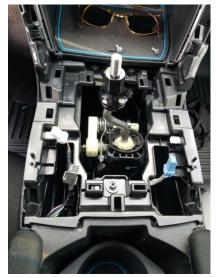
You should now have the center piece free so you can work on removing the shift boot.
