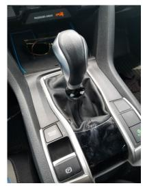
First you need to remove the shifter boot with a screw driver (usually just pops off) then you can remove the knob, most just screw off.
