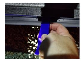
Then you are ready to remove the door panel, use a pry tool, or a wrapped screwdriver to protect the paint. Start at the bottom of the door in the center, pull gently but firmly, once you get the first couple clips free on the bottom work your way around the sides of the panel. Once you get all the clips free, pull straight up on the door panel and it should come free.
