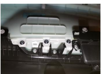
On the backside of the door panel you will find 5 screws that hold the arm rest in place, remove those 5 screws.
