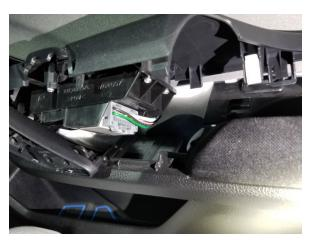
Once you get the control panel up, you will see a vertical plug, push on the tab then release them from the panel, it should be free to be removed then.
