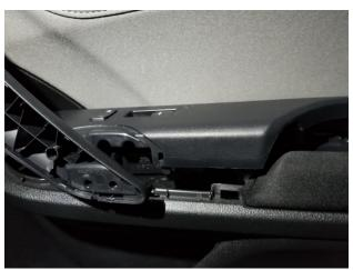
You will then be able to use a pry tool, or screwdriver, and pop up the electric window control panel, start around where the pull arm attaches and work it free.
