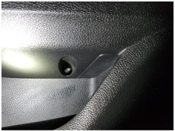
Just under the control panel and pull arm there is a phillips screw, this needs to be removed first.
