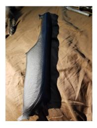
Now you are ready to slowly go around and glue all of the tabs into place. You will be using the boot fix super glue, you should wear disposable gloves, and pull the leather tight as you go around the edges and glue down the tabs. Save the long corner tabs to glue down last. Be careful not to get glue on the display surfaces, but if accidentally do, you can use nail polish remover to remove any of the glue spills when you are finished.
