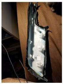
After assuring the fit, spray both sides with the spray adhesive, then carefully position the leather into place – make sure that the seam in the leather goes along the edge of your armrest. Once you have it in position, firmly press all of the surfaces into place. (Sorry I got my cats feet in the last pic (LOL))
