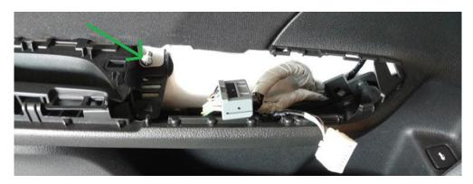
Start prying off the door panel, at the bottom-front under the speaker. Once the initial clip is popped, use your fingers to pull the panel off, popping the rest of the clips, working your way from the bottom around both sides toward the top.
