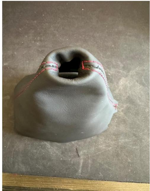
Now take your new shifter boot and fold the top of the boot in so that it can be held in by the clip of the stock shifter knob.
