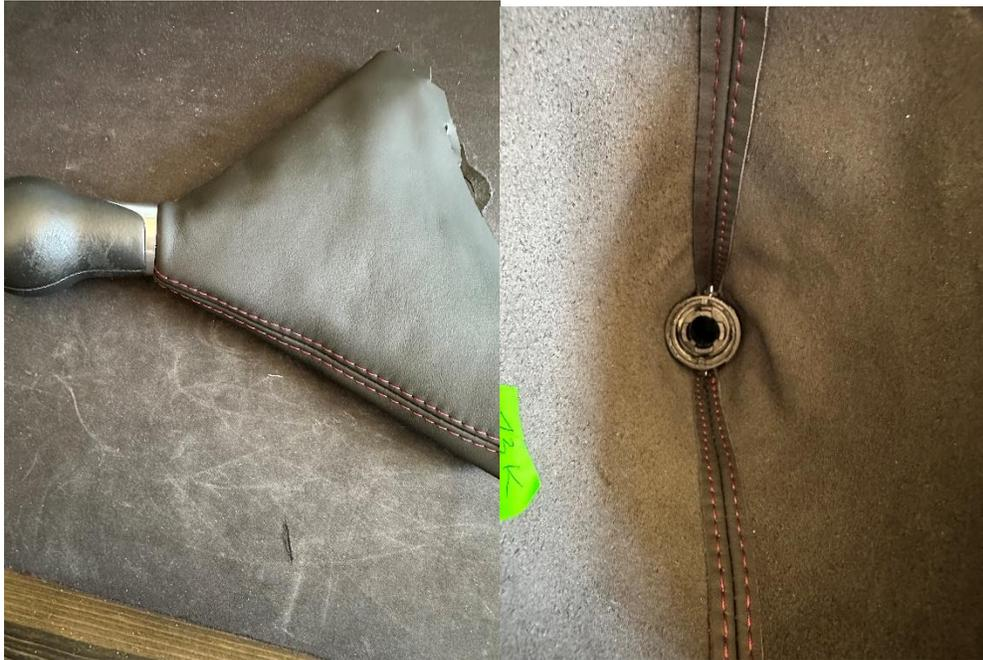
Insert the shift knob into the top of the leather boot and attach the plastic ring on the inside of the boot. Make sure to adjust the leather so that there isn't any over hanging leather and it matches how it was from the factory.
