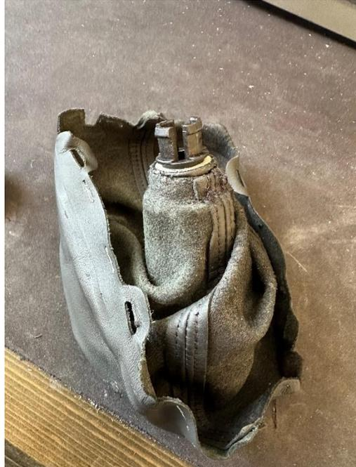
This is what the ring looks like after it has been released from the knob. It can be very difficult to remove this piece and it is easy to damage.
