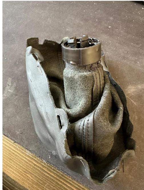
The plastic ring holds the shifter boot to the knob. This needs to be carefully pried up so that the boot can be removed. If you wish to reuse the factory shifter knob, be careful not to break this part.
