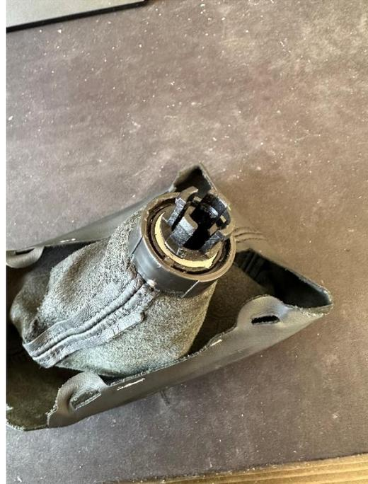
After removing the black plastic frame from the shift boot turn it inside out. The plastic frame is held in with many staples. Be care not to break it. it is near impossible to find a replacement frame, and it is required to install the shifter boot.
